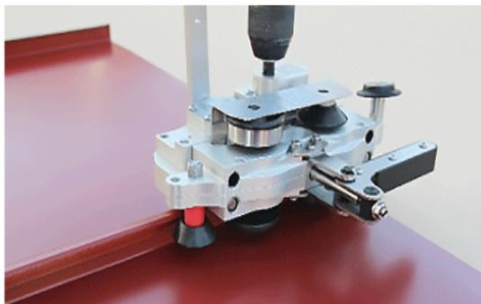
**2.** Position the ACCUSEAMER with the red marked Wheels over the Seam and start seaming.
