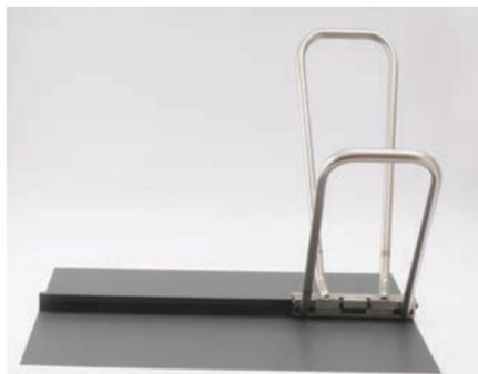
**1.** Close the beginning and the end by hand, before running the ACCUSEAMER
